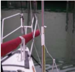
Mark to Center Mast (Measure to Cap)
