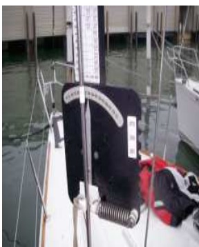
Tighten V1 = 35 (Flush Thread)
